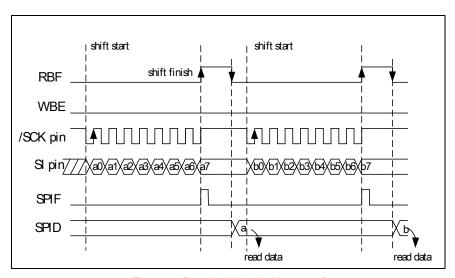
Fig. 5-15 Receive Mode (8-bit, 1 word)
